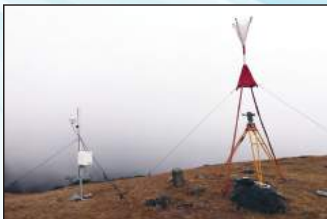
Beacon over the Wild T3 Theodolite ready for Trigonometrical leveling and triangulation and weather station during the program execution of Mt Everest Height Measurement activity.
